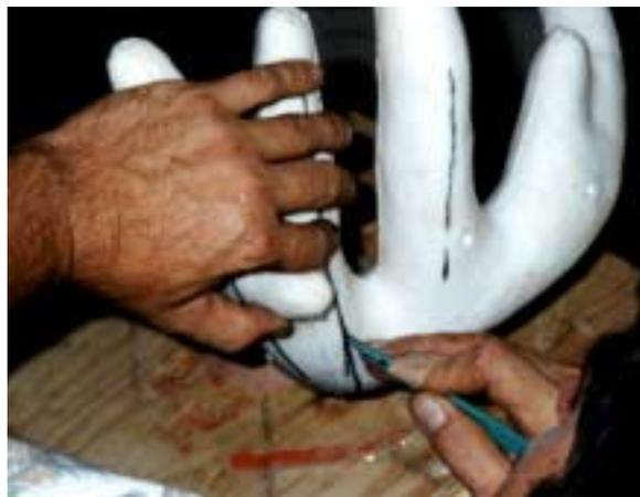
**10. Demold - Removing Antlers From Silicone:** After rubber is fully cured, remove the mother mold. You will need to make cuts in the rubber to remove the antlers. Use a marker to draw seam lines on silicone in areas that need to be cut. Do not align the silicone seams with the mother mold seams. **Stagger any silicone mold seams at least 1 inch from mother mold seams.** This will make for better registration.
