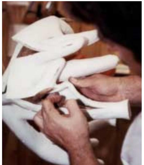
**11. Casting A Reproduction:** It is now time to mix and pour Smooth-Cast 320 liquid plastic into the finished mold. **Apply Ease Release 200 Release Agent** to the inside of the rubber mold, the inside of the mother mold and **all surfaces that will come in contact with the liquid plastic**. Reassemble the rubber mold into the mother mold and loosely affix bolts. Do not tighten bolts yet.
