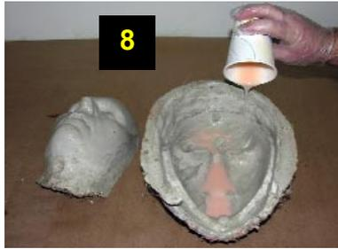
8. The blend is then poured into the the lowest part of the mold, allowing the liquid to seek its own level.
