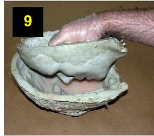
9. The face plug is then pressed into the mold. A mold strap is then used to secure and pressurize.
